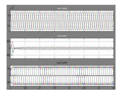
Fig. 3.5:Source Voltage, Source Current, Load Current with FLC H.Harmonic spectrum of phase-a source current with FLC
