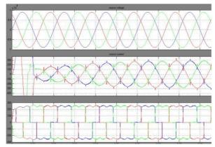
Fig 3.2:Source voltage, current and load current with D-STACTOM
