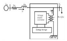
Fig 2.1: Schematic Diagram of a D-STATCOM
