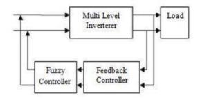
Fig2.3: Block diagram of Feedback controller
