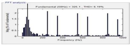
Fig.3.4: Harmonic spectrum of phase-a source current with DSTATCOM
